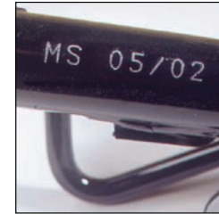
Marking after surface treatment
