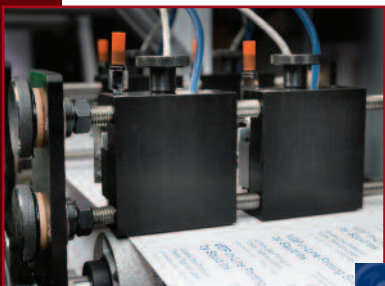
Printhead mounting brackets allow accurate print placement at the turn of a knob.
