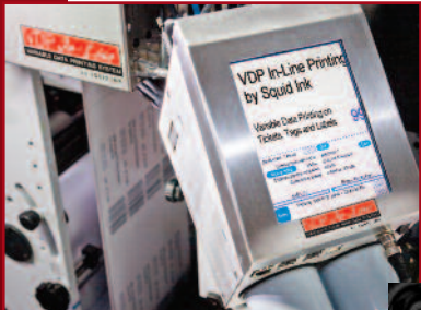
Color touchscreen display offers ATM-simple software for message creation and recall.
