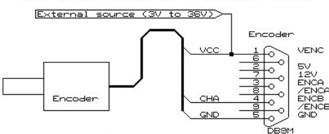
External power source encoder single channel NPN/ PUSH/PULL encoder
