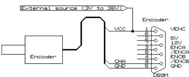
External power source encoder single channel PNP encoder
