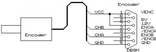
12 VOLT encoder double channel NPN / PUSH/PULL encoder
