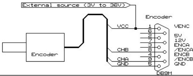
External power source encoder double channel PNP encoder
