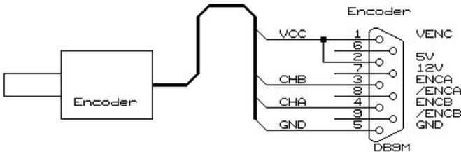
5 VOLT encoder double channel NPN / PUSH/PULL encoder
