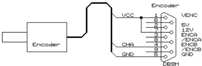
12 VOLT encoder single channel NPN/ PUSH/PULL encoder
