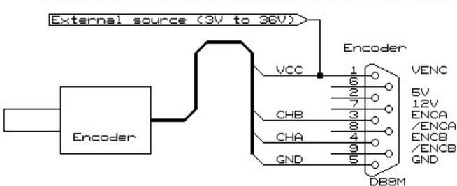
External power source encoder double channel NPN / PUSH/PULL encoder
