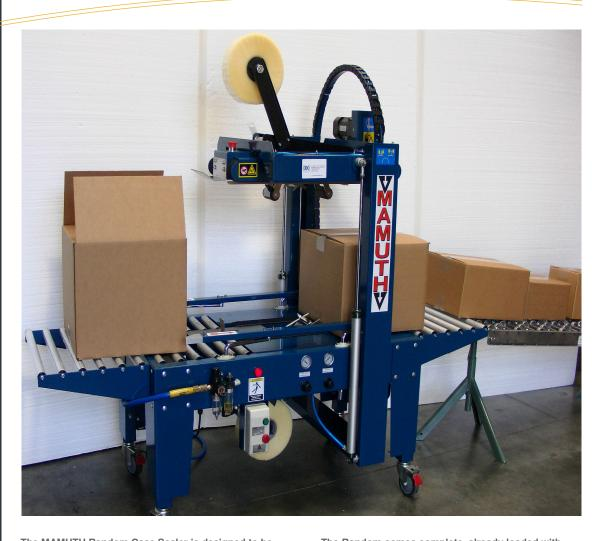
The MAMUTH Random Case Sealer is designed to be the most helpful piece of equipment on your production floor. There is no changeover required to re-configure your case sealer to accommodate constantly changing box sizes when you have the Random. It is a very rugged, heavy gauge system with top and bottom belts to securely and powerfully turn your case sealing into a quick, complete, inexpensive and almost effortless part of your production process.
